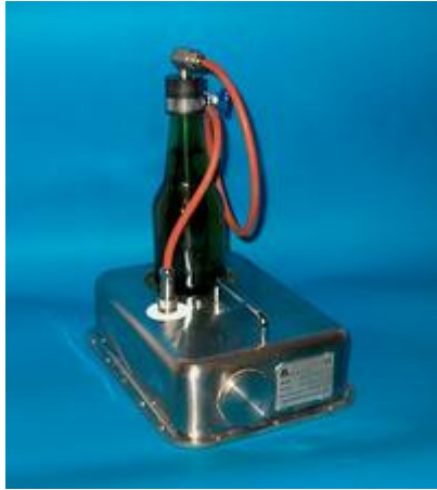
PRU-2010 with temperature probe and rubber adapter for bottle
