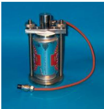
Combined probe for temperature and pressure with can's adapter
