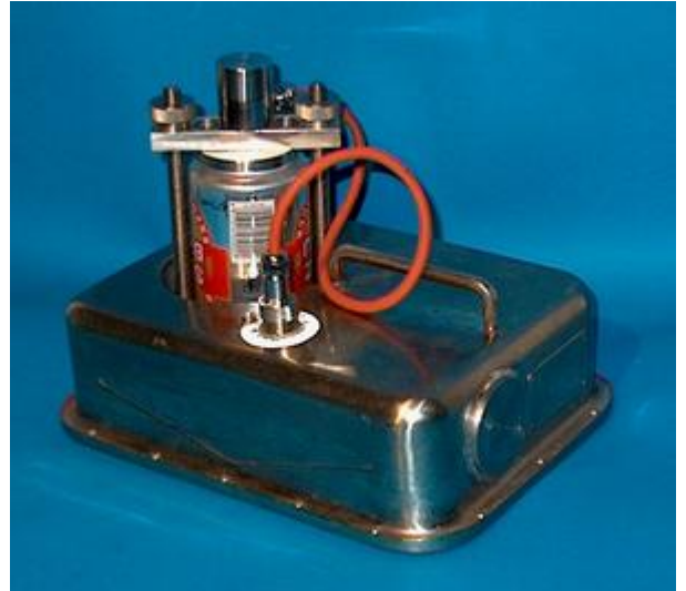
PRU-2020/P - combined probe for temperature and pressure and can's adapter
